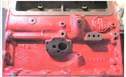
22290 block with date code, plain diamond & MG logos. Photo by Alasdair Enticknap
