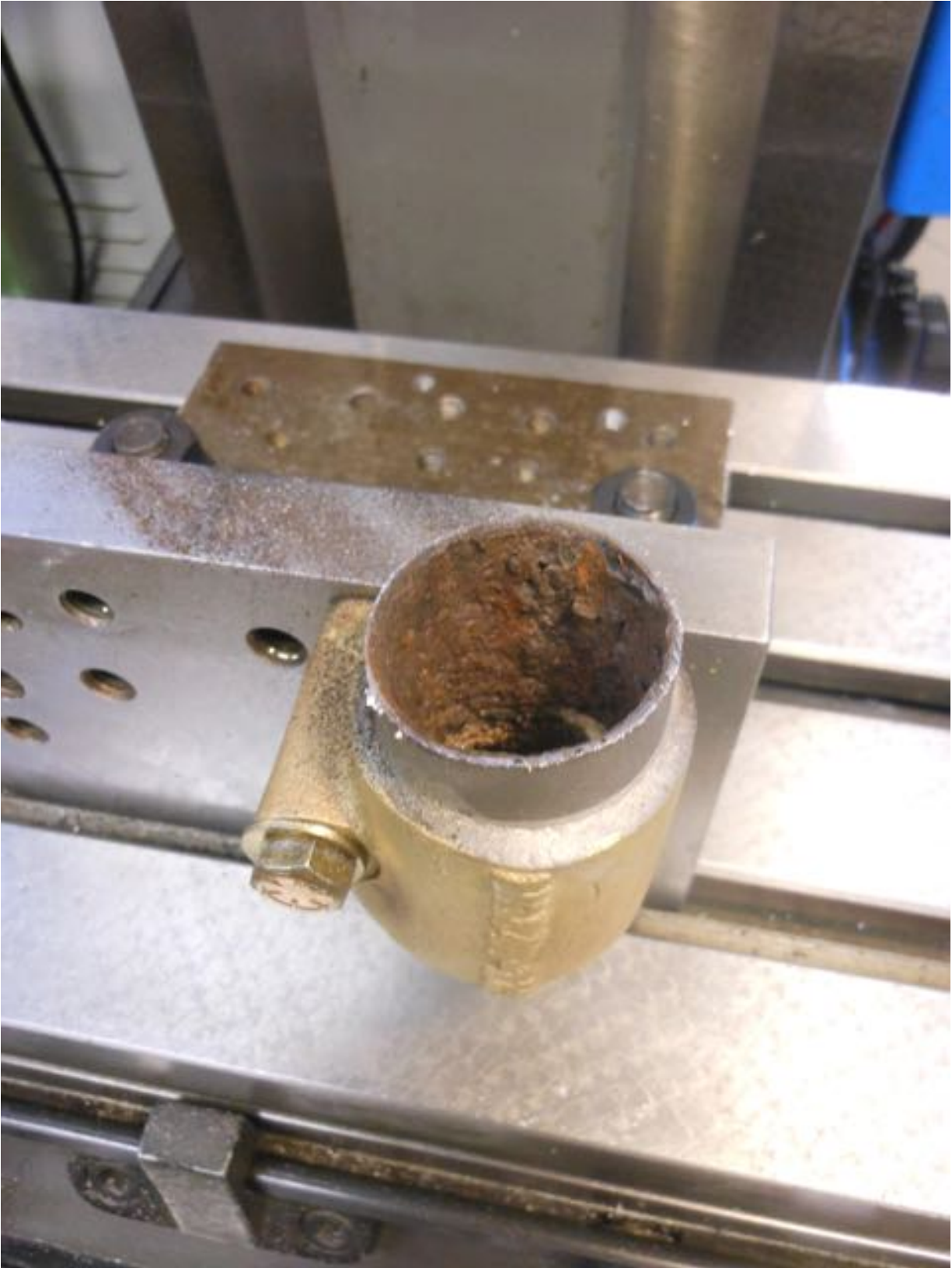
The tube can then be bored out removing all evidence of past
