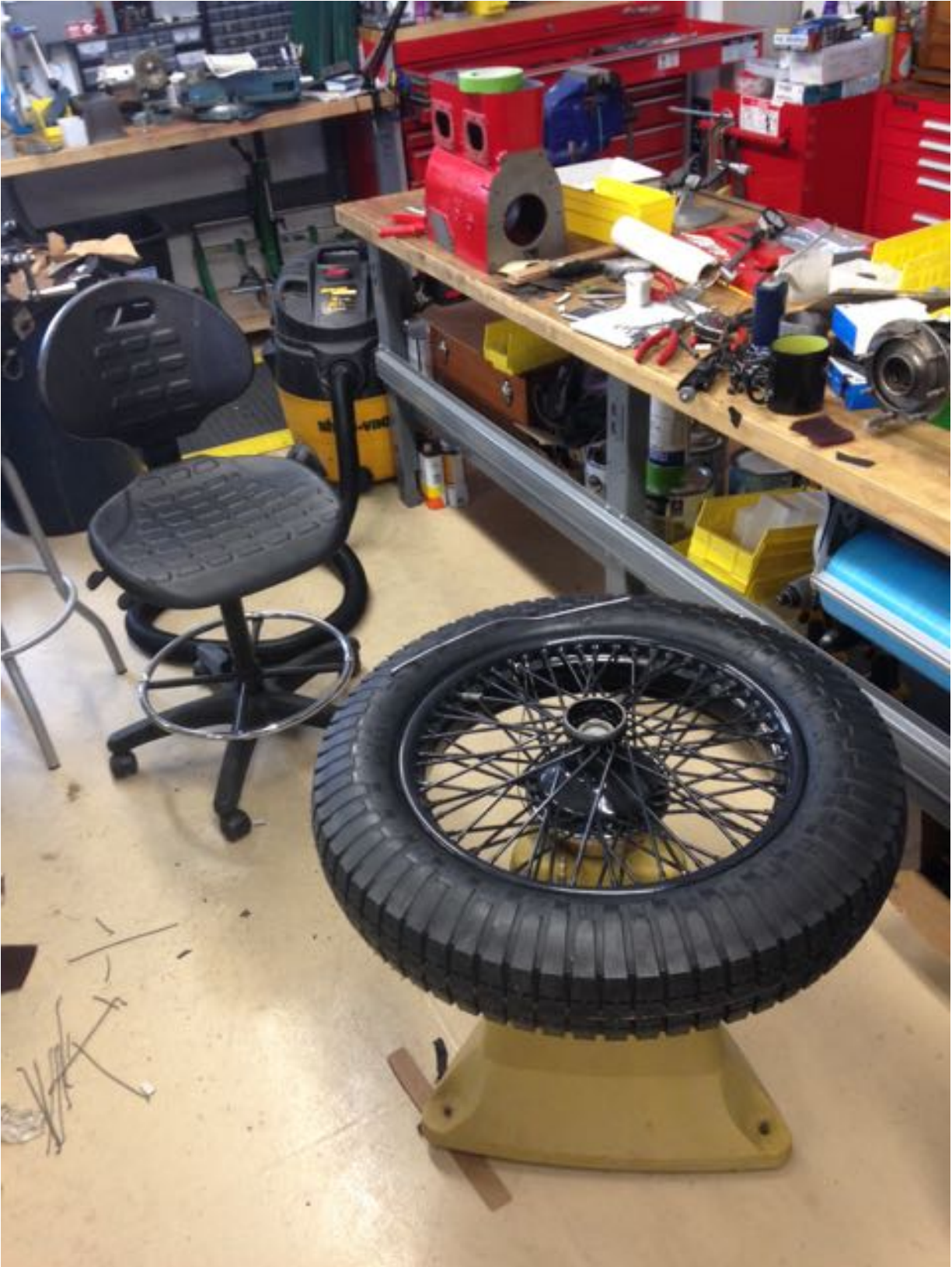
The object is to use the lead wire wrapped around designated spokes to counter a combined imbalance in the wheel and tire.
