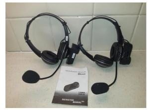
I had a pair of lightweight telephone headsets of the type that are often used in call centres, I removed the tiny earpieces and replaced them with the intercom's speakers. The intercom unit was attached to the side of the headset.
