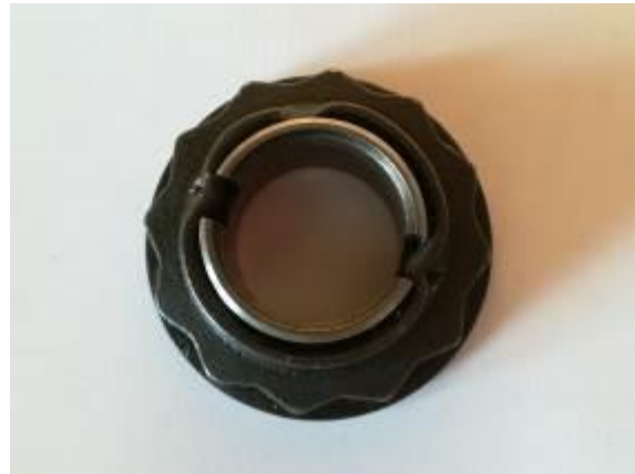
Top view of the (peened) nut -
