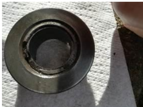
And the nut, from below (see matching shear)
