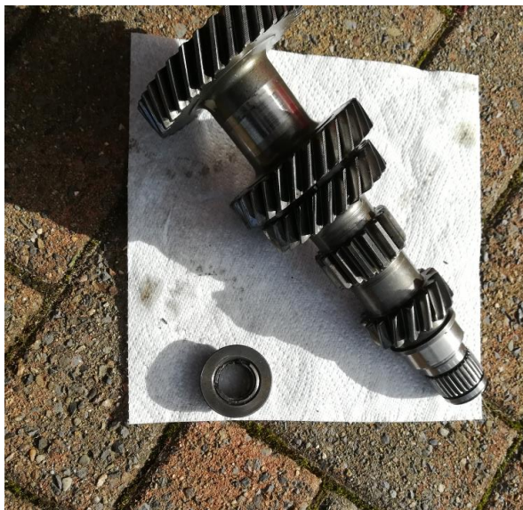
The broken cluster, with sheared nut and tube below (left)
