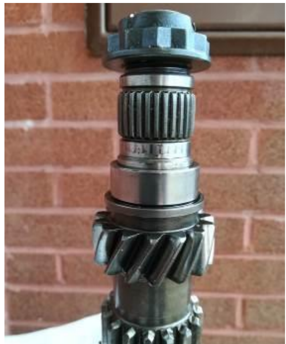
How the cluster SHOULD look, with nut (balanced!) in place (right)
