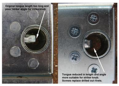
In the graphic, on the left is shown the lock tongue length and strike angle as originally supplied, and the modified one on the right. In the modified form, the lock tongue is reduced in length by 2mm and the angle has of the tongue been reground to create a more parallel strike angle to that of the door striker knob. There is still ample projection of the tongue in both the first and second holes of the door striker. It works beautifully now. The supplier has been informed.
